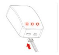
The battery comes 30% - 50% charged from the factory, but it needs to be fully charged (12.4-12.6 volts) before use.
