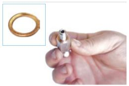
Install the copper washer from Step 4 onto the new fitting's threads. Continued...
