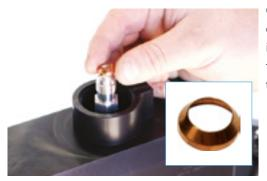
Carefully place one of the included copper flare seals onto the fitting.
