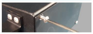
Ensure the unit is powered off. Using a standard 1/8" allen wrench, unscrew each of the four screws holding on the removable base-plate on the bottom of the body. Once the base-plate is removed, you will be able to access the battery.
