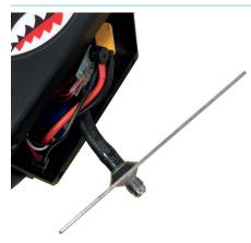
Attach the freshly disconnected end of the hose to the barb on the conversion kit bottom plate.
