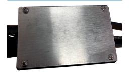
Remove the four screws from the bottom plate and remove the plate.
