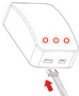
The battery comes 30% - 50% charged from the factory, but it needs to be fully charged (12.4-12.6 volts) before use.
