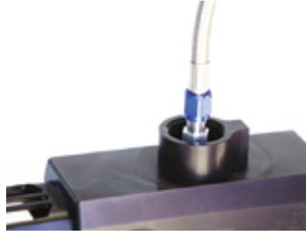
Tighten the fitting using an AN wrench designed for -6AN fittings, or a standard 11/16" open-ended wrench. Do not over-tighten, as all parties involved are aluminum.
