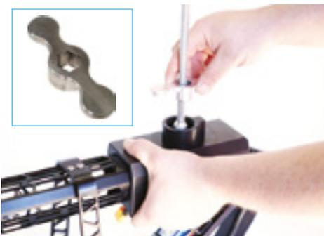
Use the included hex fitting tool to loosen the pipe.
