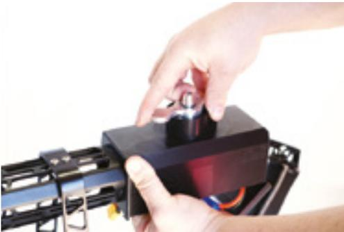
Use the hex fitting tool to tighten the new fitting as well as you can by hand using the tool only.
