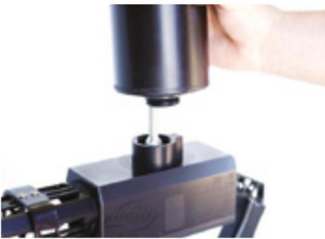
Check the fuel canister to make sure it does not have any fuel in the tank before removing it. Once fuel tank is verified as empty, unthread the fuel canister from the XM42-M body.
