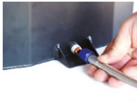
Install a copper flare seal onto the backpack's fitting. Thread the other end of the braided hose onto the backpack's fitting and tighten securely.
