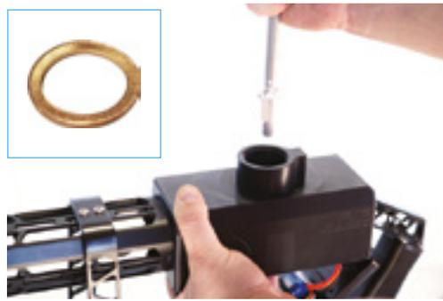
Unscrew the pipe the rest of the way by hand. Retain the copper washer from the pipe's threads.
